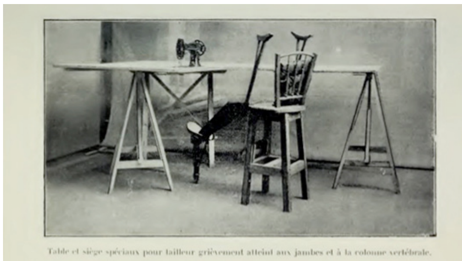
Image 2. Sewing-table made at Port-Villez for disabled tailors. The table enabled a tailor with an injured pelvis and a paralysed left leg to work at a sewing-machine without straining his body. 16 (Illustration from La Rééducation Professionnelle des Soldats Mutilés by Léon de Paeuw, 1917 © Universiteitsbibliotheek KU Leuven).
